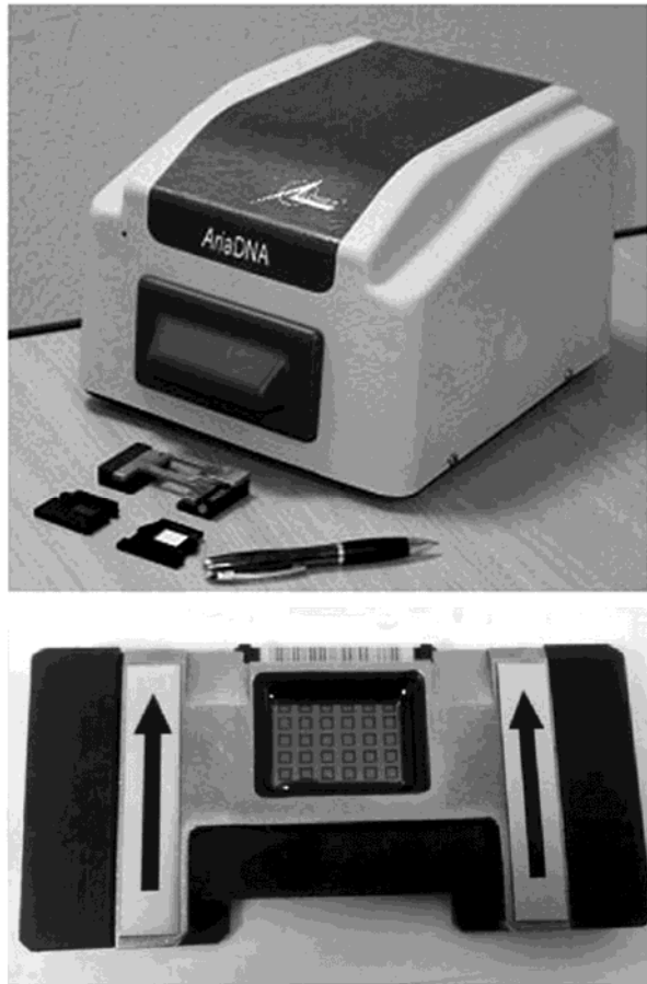
Fig. 1. AriaDNA ® real-time microarray amplifier with two qPCR microarrays and a holder (top) and a standard 30-well microarray in a holder (bottom).
